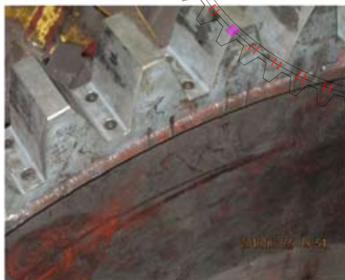
New Teeth Ring secured to the Flywheel with Bolts.
