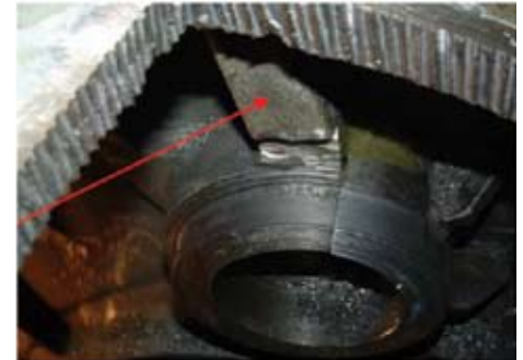
The fitted Inserts O/D has been machined.
