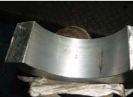
The damaged Housing was prepared to accept the new pre machined insert.
