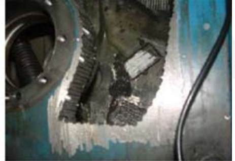
The Flywheel was removed to enable two sections of the Engine to be cut out to access the damaged Housing.
