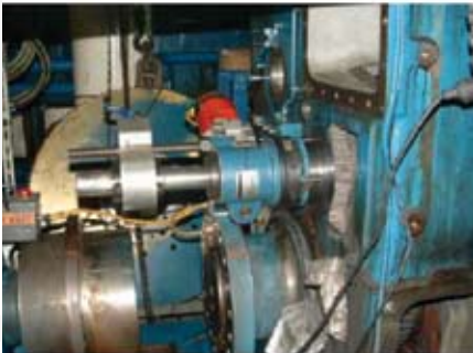
Mounted portable boring bar for machining outer collar of insert and boss material.
