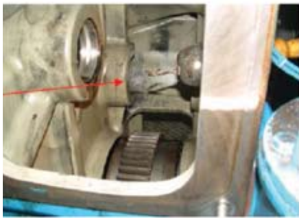
Gears removed exposing the damaged Housing.
