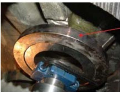
Steel Ring fitted prior to machining.
