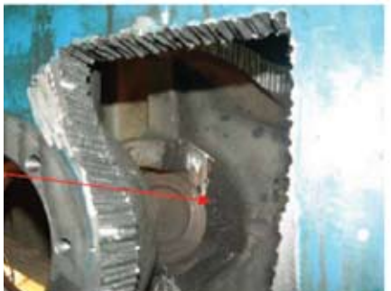
The removed castings taken from the two apertures were retained for use upon completion of the repaired Housing.
