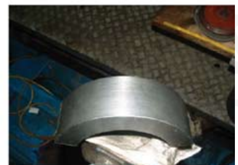
The damaged Housing was prepared to accept the new pre machined insert.
