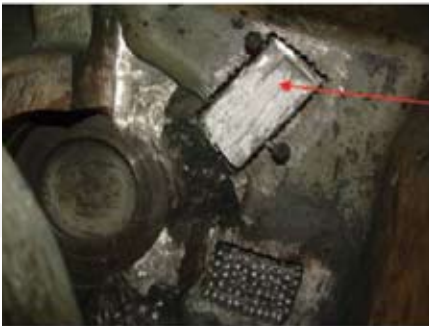
Steel inserts were inlaid into the casing, becoming integral with the parent casting.
