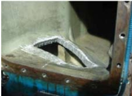
The removed castings taken from the two apertures were retained for use upon completion of the repaired Housing.
