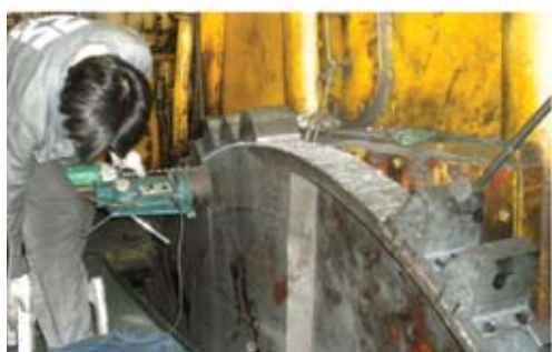
All Teeth were removed by drilling.
