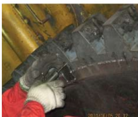
All Teeth were removed by drilling.
