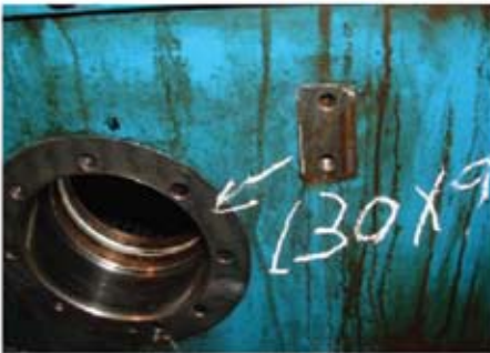
The Flywheel was removed to enable two sections of the Engine to be cut out to access the damaged Housing.
