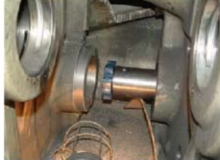
Mounted portable boring bar for machining outer collar of insert and boss material.
