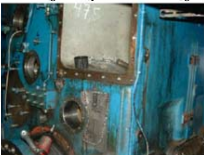
Steel Ring fitted prior to machining.
