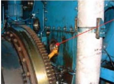
The Flywheel was removed to enable two sections of the Engine to be cut out to access the damaged Housing.
